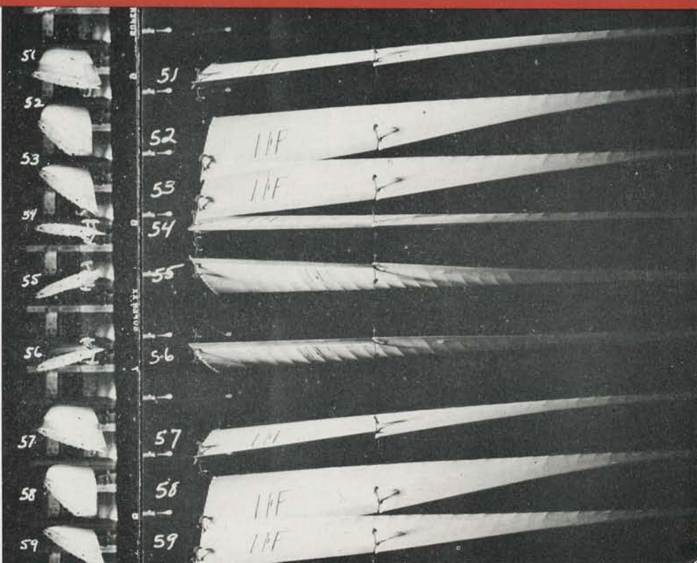
TOP OF PAGE —This is how a wing looks to a flutter man. The vibration of every section is recorded in lines on a graph by means of a series of electric strain gages. ABOVE —On a special B-17, Ellis Levin and John Shepard take flutter readings. BELOW —This section of movie film, made at Massachusetts Institute of Technology, reveals wing flutter in an airplane model that is undergoing a wind tunnel workout.
